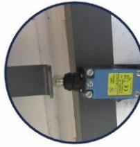
*All our kilns are equipped with an Element Cut-Off switch, which automatically deactivates the electricity-carrying element when the kiln door is open. This feature is integral to ensuring safety.*
