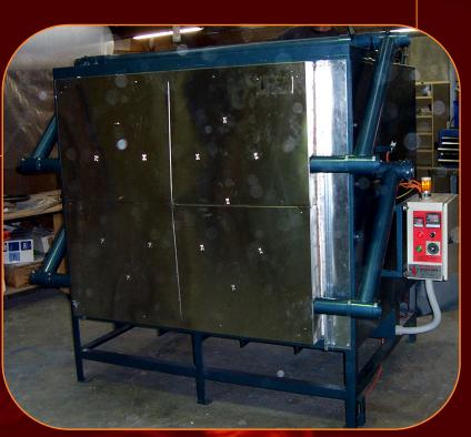
A vertically opening door keeps hot surfaces away from the operator for safety and ease of loading.
